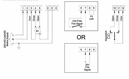
1. Power Supply: Connect a 230VAC supply to terminals as shown.
