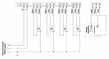
Wiring for Individual Tube Motor Control...
