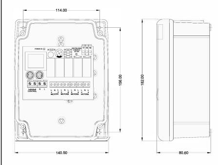
Overall Dimensions: 140.50×182.00×80.60mm Mounting Hole Dimensions : 114.00×156.00mm
