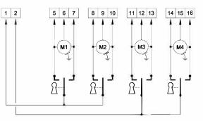
Note:- Connect ALL tube motor earth wires together and wire to ground.
