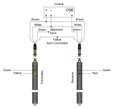
Note: Reverse the brown and white cables on the transimitter to turn off the blanking function.
