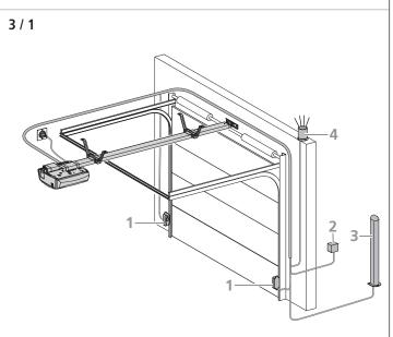
This is just an example of a door system. The details can vary according to the type of door and the associated equipment. The system shown comprises the following components:
