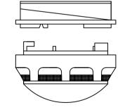
Twist clockwise to lock and twist anti-clockwise to unlock
