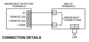
1. Connect 'ZONE+' from Smoke/Heat Detector to `L1`on the EMC-3C. Connect '0V' from Smoke/Heat Detector to 'L2' on the EMC-3C
