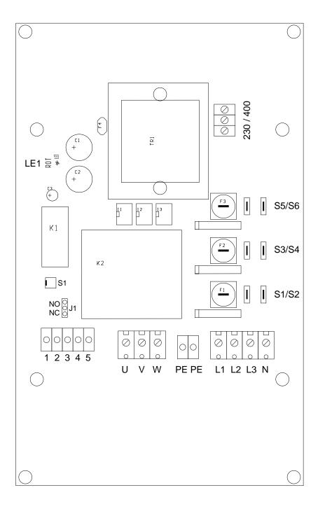
Key: L1, L2, L3, N, PE: terminal block
